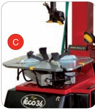
**EN** **SELF-CENTERING TURNTABLE:** System able to lock rims from 10" to 25" without adapters and adjustments: internal clamping capacity 10"-22", external 13"-25". It employs unique rod geometry to ensure constant and even clamping power throughout all rim diameters.
