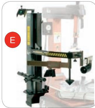
**(EN) UNIVERSAL PNEUMATIC DEVICE UPH & BPS (OPTIONAL):** Universal auxiliary device UPH, which assists the operator to easily mount and demount particularly tough or low profile tyres such as «Run-Flat». This patented system allows to handle the second tyre bead without using the lever, thus avoiding any risk of rim damaging. Usually supplied complete with the second floating presser BPS.
