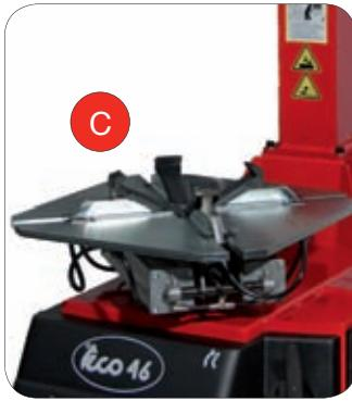
**(EN) SELF-CENTERING TURNTABLE:** System performing a total clamping capacity from 10" to 25" for TECO 46 and from 11" to 27" for TECO 48 without adapters and adjustments. It employs unique rod geometry to ensure constant and even clamping power throughout all rim diameters.
