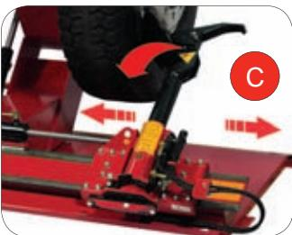
**(EN)** **VERSION TECO 540 S:** Automatic translational movement of the tool-holder carriage and hydraulic lifting of the tool-holder arm controlled by the on-purpose control unit. The rotation of the tools is manually achieved through an on-purpose unlocking pedal.
