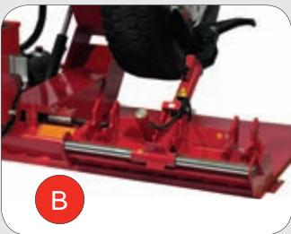
**(EN)** **VERSION TECO 540 N:** Fixed tool-holder carriage and manual lifting and traversing of the tool-holder arm, which can be secured in 3 different working positions. The rotation of the tools is manually achieved through an on-purpose unlocking handle.
