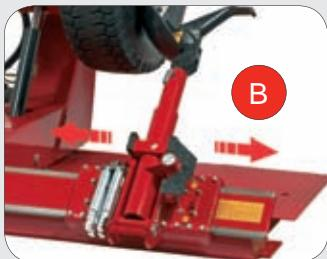
**(EN) VERSION TECO 560 N:** 1-speed automatic translational movement of the tool-holder carriage controlled by the on-purpose control unit and simultaneous to the automatic chuck movement. Lifting and rotation of the tools are manually achieved through an on-purpose unlocking device.
