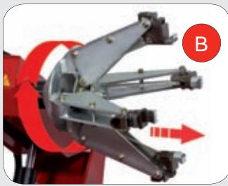
**(EN) SELF-CENTERING CHUCK:** The hydraulic chuck has working capacity from 14" to 44" which can be also extended till 60" using the optional SE-580 extensions. It performs a 2-speed rotation in both directions and a 2-speed automatic traversing simultaneous to tool-holder carriage translation.
